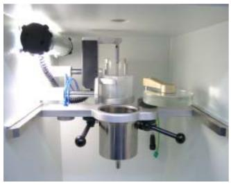
The compression funnel is replaced only with the normal funnel and connected with 3 plug-type coupling units. The conversion is complete. A job of seconds.
